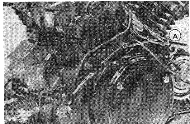
A. Sealant Coated Bolt, 30 mm long
